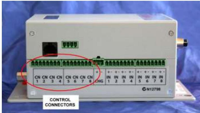
Each control provides normally open relay contacts rated to 30V, 1A resistive loads. External **protection diodes must be installed** when driving inductive loads such as power relays.
