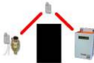
EXAMPLE: While each leg of the transmission is line-of-sight a repeater can be used to change the direction of the signal
