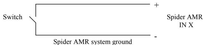
2. "ANALOGUE" type accepts an analogue voltage from 0 – 2.5V. The following diagrams show wiring details for most common sensor types.
