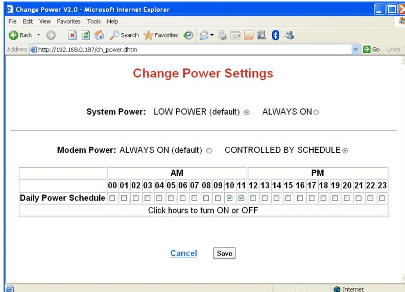
To control the hours of the day when the modem is on, simply click on the relevant box. In the example above, the modem will be on between 10:00 AM and 11:59 AM every day.
