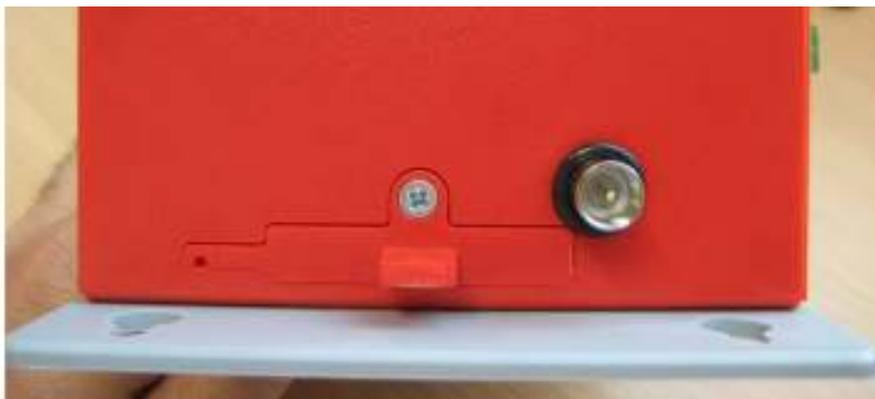
2. By looking through the slot, you will see the SIM card slot with a black locking lever to the left of it. Holding the SIM card level with the locking lever, gently push the SIM card into the exposed slot until it locks in. The notched end should be inserted first, with the gold contacts facing up – as shown in the illustration.
