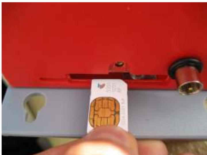
**IMPORTANT:** You should feel slight resistance while pushing the card into the slot. If you do not or you can freely move the SIM from side to side by more than 1 mm you have missed the slot. You must remove the SIM and try again!
