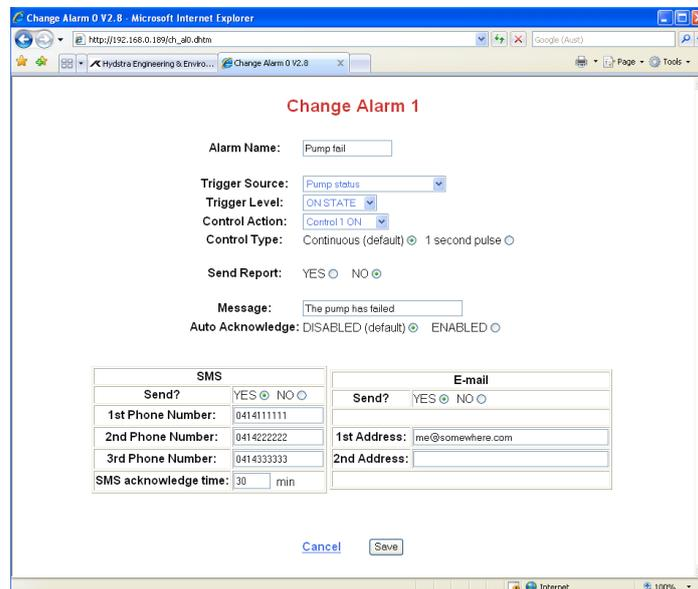
The "SMS acknowledge time" is the period of time (in minutes) during which an alarm must be acknowledged and to stop the Spider from sending SMS to the next number on the list. It can be set to 0 to 60 minutes.
