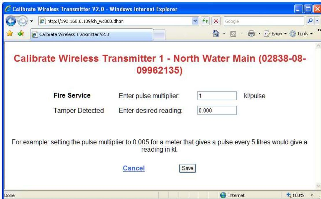
Two calibration parameters are available for every input connected to the current transmitter.
