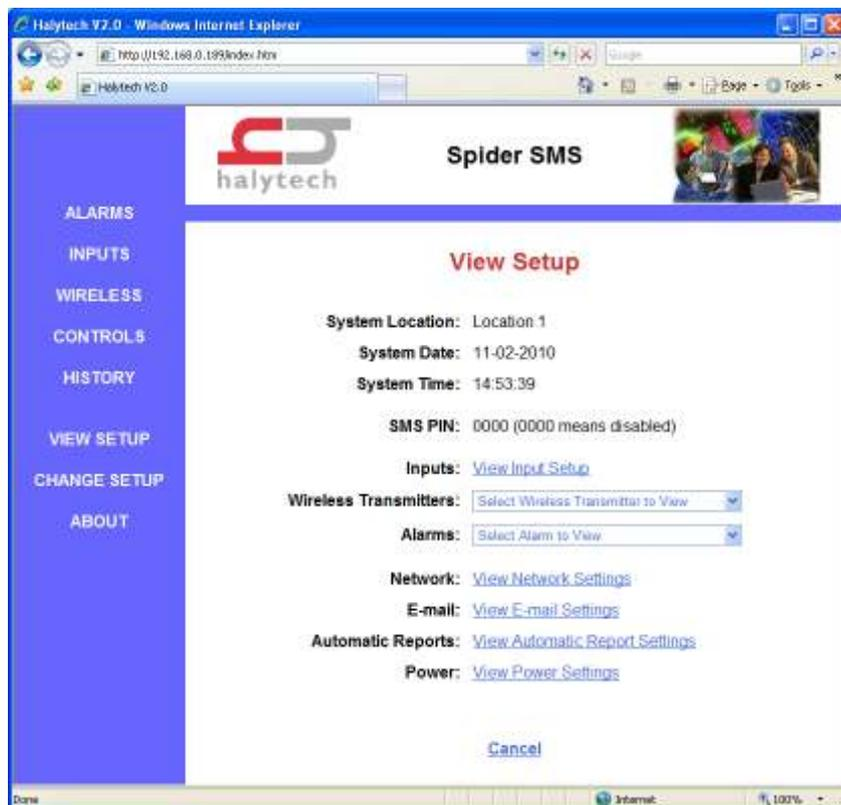
This page allows inspection of all Spider AMR programmable parameters, without making any changes.
