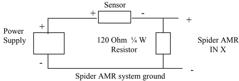
(ii) **4-WIRE 0 - 20 mA and 4 - 20 mA** current loop sensors require an external 120 Ohm, ¼ W resistor:
