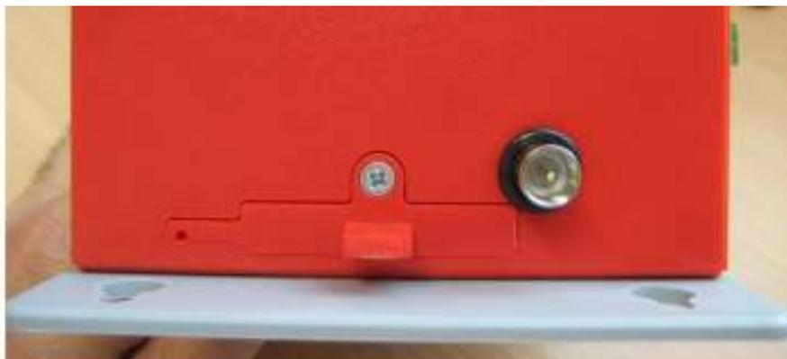
2. By looking through the slot, you will see the SIM card slot with a black locking lever to the left of it.
