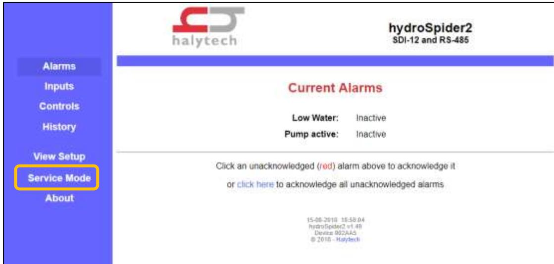
The service mode is intended to allow field personnel perform diagnostic tests, recalibrate sensors and reset the unit’s time, without being granted access to change the unit’s setup.
